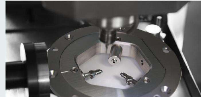
Universal disc grip of 98 mm diameter for metal milling machines to position fast and precisely 3 pre-milled abutment blanks with engagement on the back side of the implant connection.
