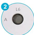
2 Select stopper according to drill diameter (rows), and drilling depth (columns)
